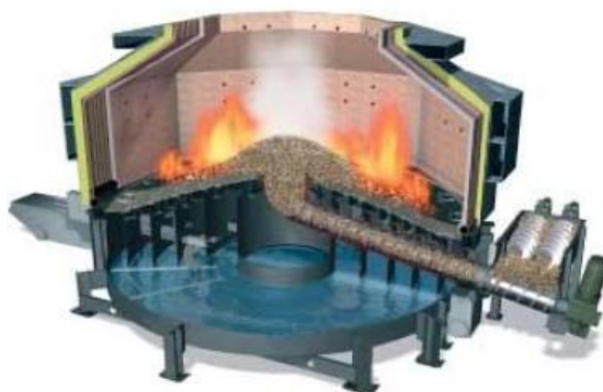
Figure 7-3: Central lower biomass feed system 18
