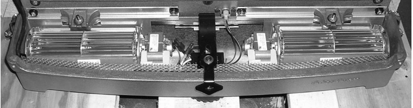
Photo 30 – Blower System (Ash Lip Cover Removed)
