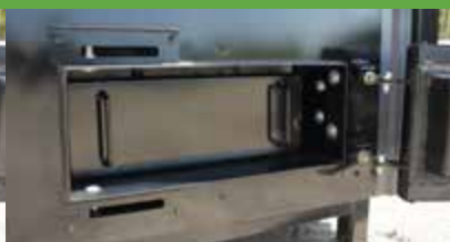
Secondary Combustion Chamber Heat Shield
