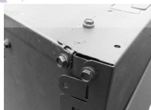
Step 1: Remove two screws from the top and side of the unit. Bend the side bracket securing tab over the edge of the unit and secure. Secure bracket to the top through the clearance screwhole.
