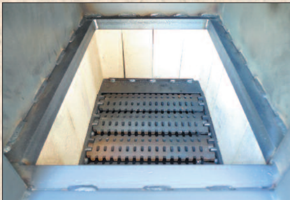
Inside Fire Box.
