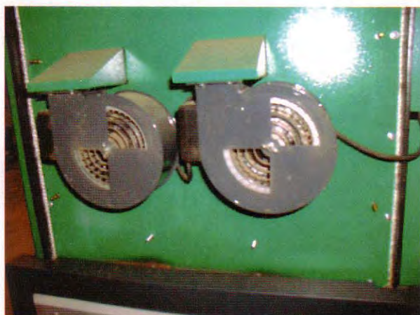
Fig. 3: - combustion air fans
