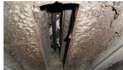
Stainless burner tube with 70 ports – as viewed from secondary chamber
