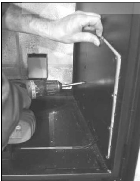
Figure 13: Removing Access Cover.
