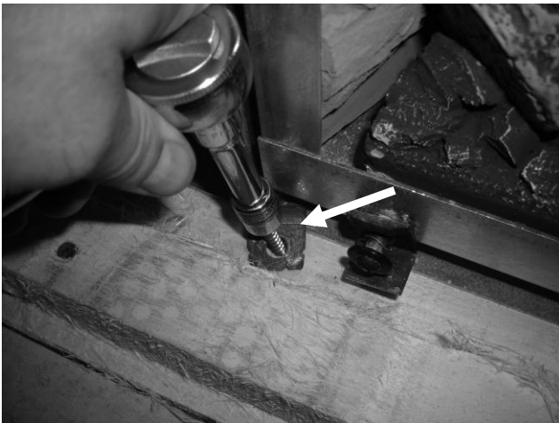
Figure 11 – Shipping Clip Detail
