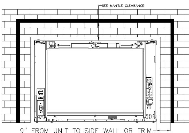
Figure 17 - Minimum Side Trim Clearances
