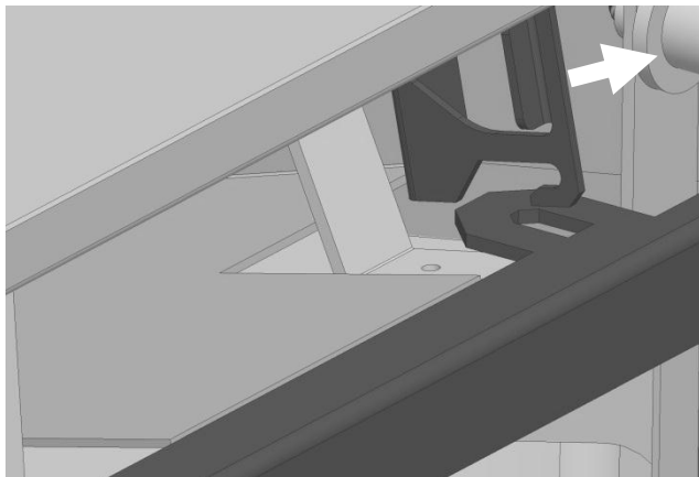
Figure 12 – Glass Frame Upper Mounting Detail
