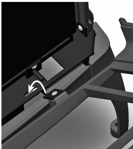
Figure 11 – Front Panel Retaining Slots
