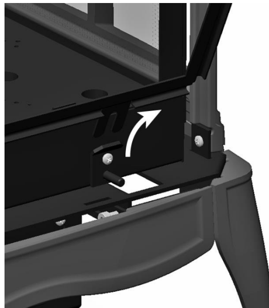
Figure 13 - Lower Mounting Stud/Spring Detail
