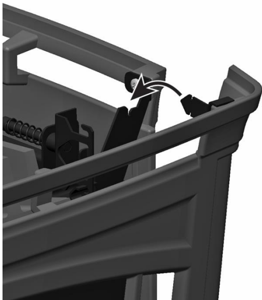
Figure 10 – Front Panel Mounting Tang Detail
