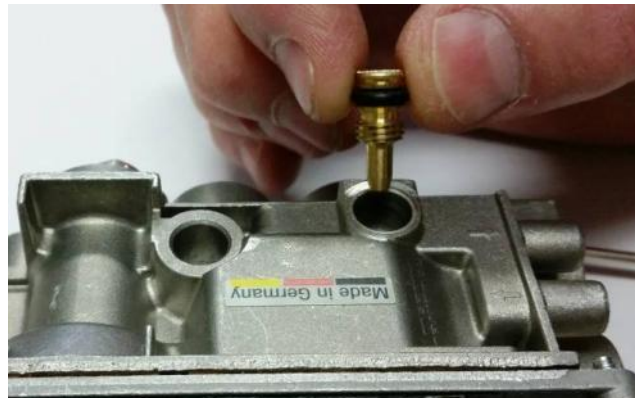
Figure 23 – NG Low Flow Screw Removal
