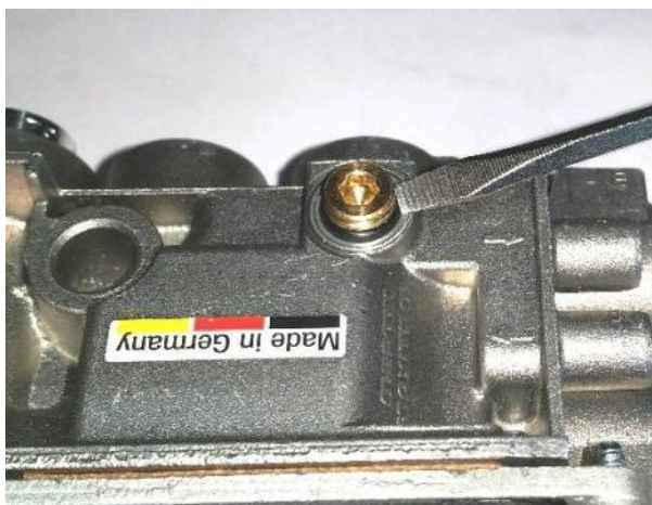
Figure 22 – Low Flow Orifice Removal – O-ring
