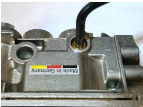
Figure 21 – Low Flow Orifice Removal
