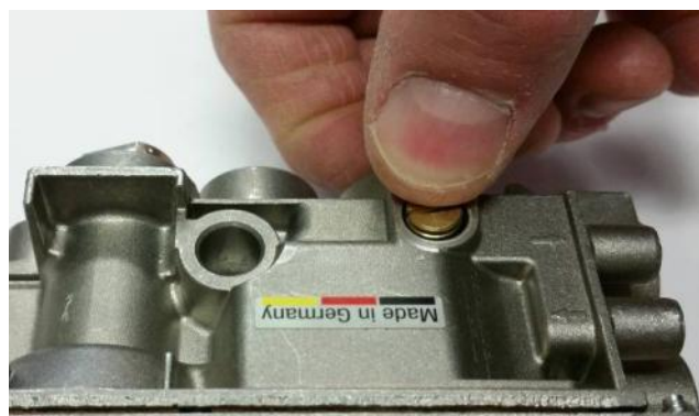
Figure 23 – NG Low Flow Screw Removal
