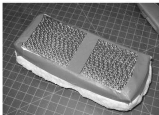
Figure 20 - Installing Gasket on Catalyst
