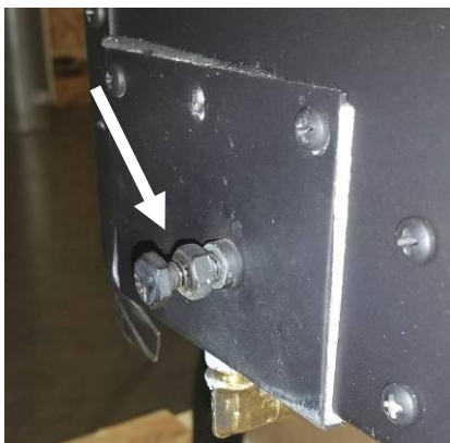
Figure 33 – Air Shutter Closed
