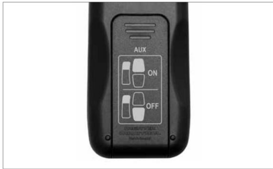
Figure 39 – Aux Burner Control Instructions
