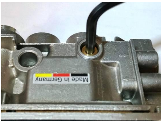
Figure 23 – Low Flow Orifice Removal
