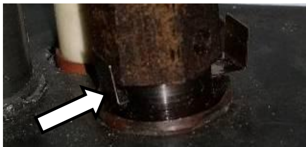
Figure 29 – Loosen Tower and Slide Pilot Gate to Rear of Pilot Tower (LP position)
