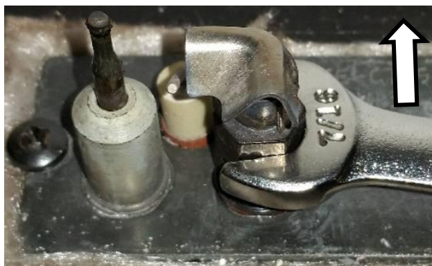
Figure 28 – Pilot in NG (Pilot Gate forward)
