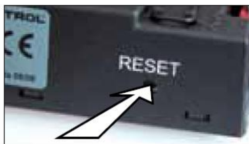
Figure 37 – Receiver Reset Button Location
