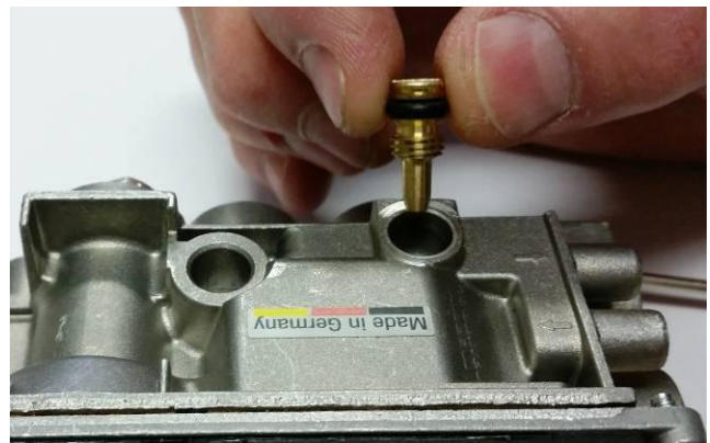
Figure 25 – NG Low Flow Screw Removal
