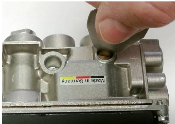
Figure 27 – Tighten LP Low Flow Orifice
