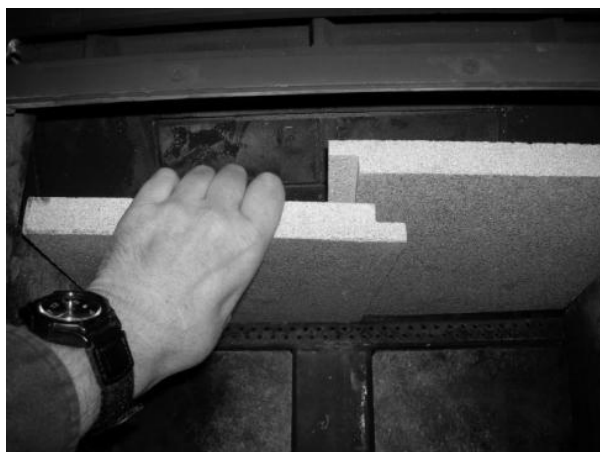
Figure 16 - Removing/Replacing the Baffle for Inspection
