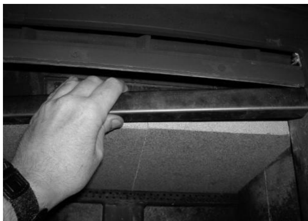
Figure 16 - Removing/Replacing the Baffle for Inspection
