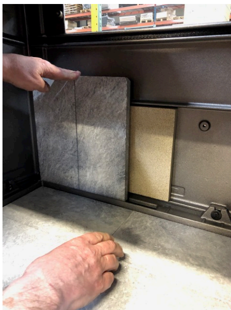
Photo 1. Insulation panel placed behind left rear refractory stone.
