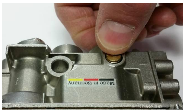
Figure 24 – NG Low Flow Screw Removal
