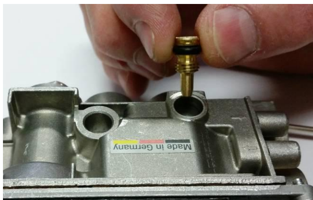
Figure 24 – NG Low Flow Screw Removal
