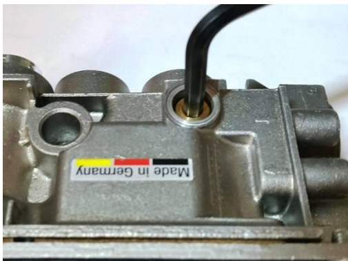
Figure 22 – Low Flow Orifice Removal
