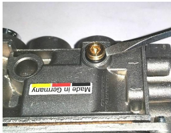
Figure 23 – Low Flow Orifice Removal – O-ring
