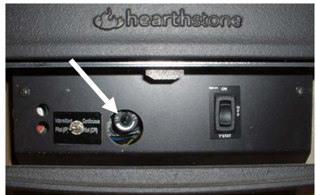
Photo 39 – ST Valve Output Control
