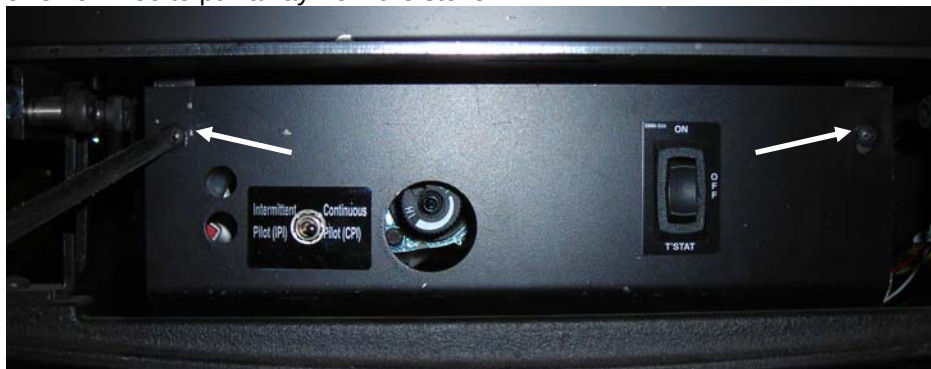
Photo 15 – Modesty Panel Removal
