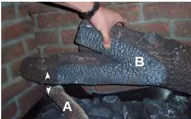
Figure 88: Log B Position
