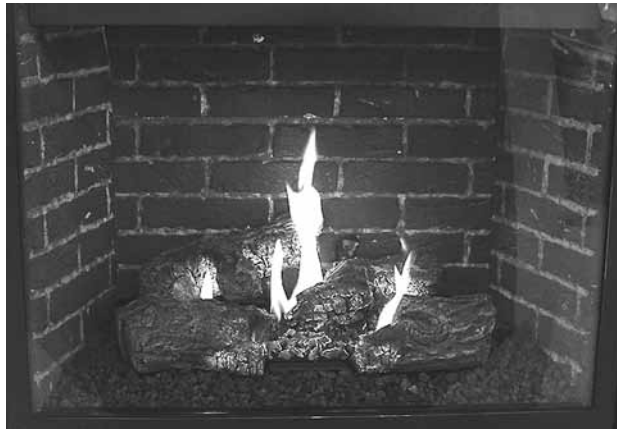
Figure 13 - Burner Flame Appearance Model SLDVT-40
