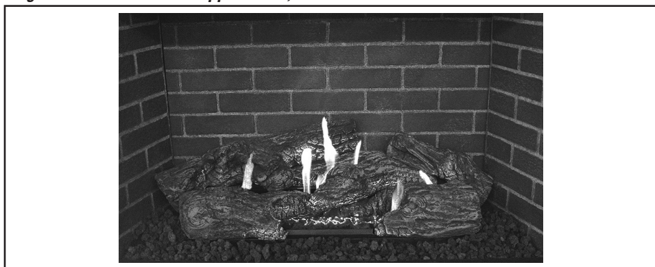
Figure 39: Burner Flame Appearance, SLDVT-45
