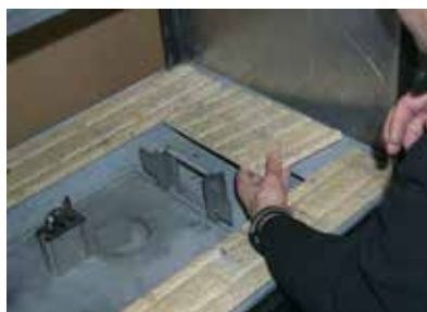
Remove Left & Right Side Base Brick Panels
