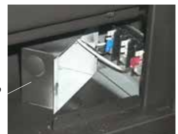
Remove cover to access Terminal Block
