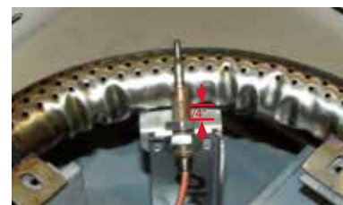
Diagram 4 - correct thermocouple position
