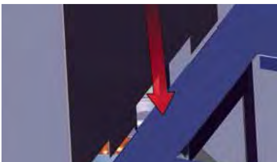
Diagram 2 - Lower tabs on panel aligned with base
