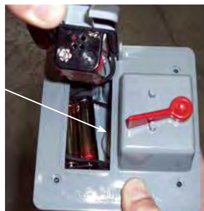
Slide 1st battery pack to the right.
