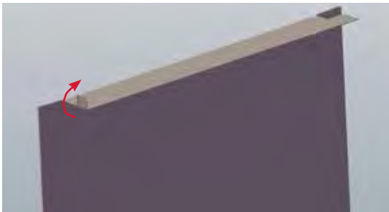
Diagram 1 - Bend tabs to 90°
