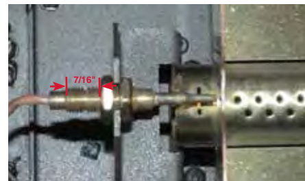
Diagram 4 Correct thermocouple placement
