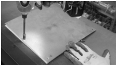
Step 1: Remove the two (2) screws holding the top vent cover plate and gasket.
