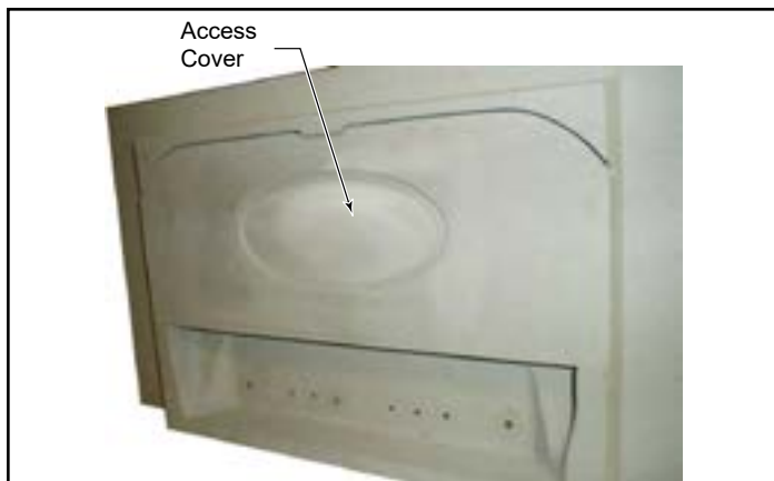
Figure 5.9 - Remove access cover.
