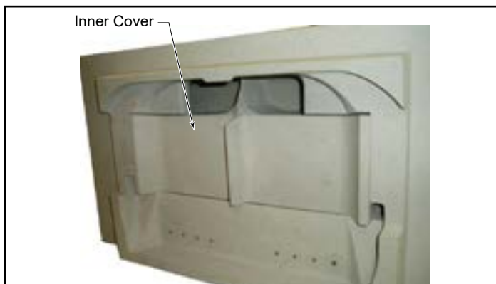
Figure 5.10 - Remove inner cover.
