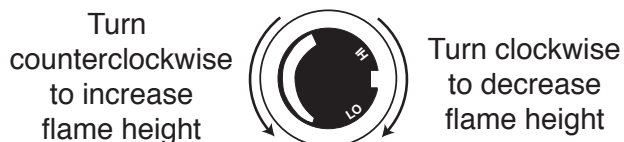
Fig. 56 Flame adjustment knob for SIT valve.
