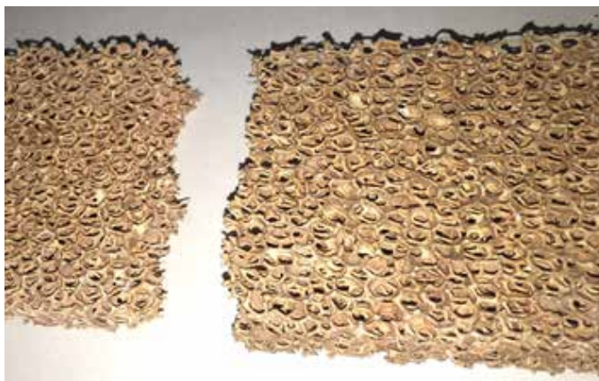
Combustor Problem - Broken Combustor
