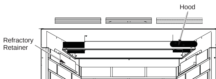
Figure 20 - Installing PureFire Hood
