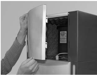
Fig. 134 Removing the cladding
