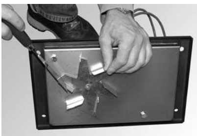
Fig. 132 Cleaning the blower wheel
