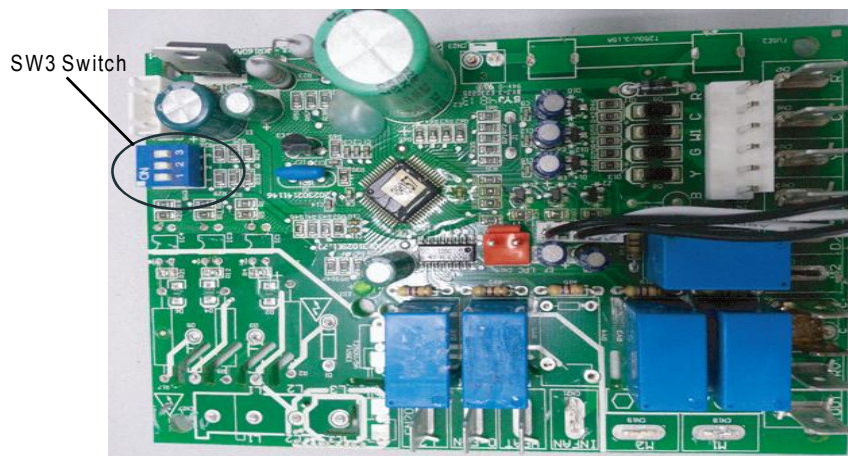
Fig.11 SW3 Switch Location in the PCB Board
