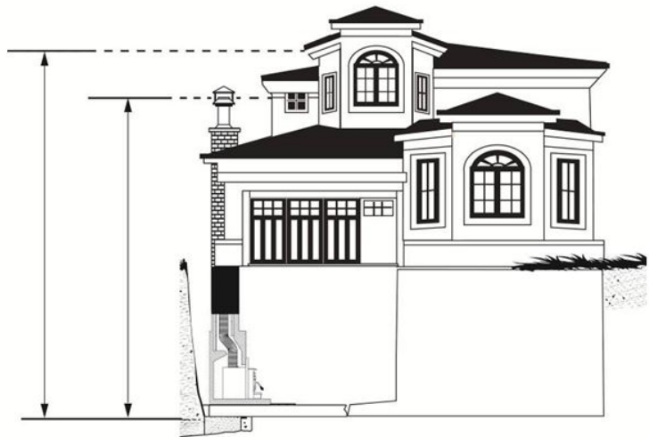
Figure 32: Chimney location in the house
